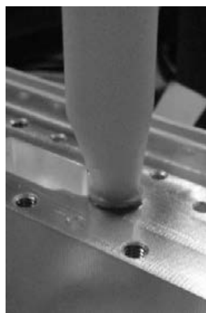
Fig. 2. OCP measurement on a complex shape.
