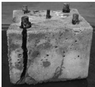
Figure 1.- Aspect of the mortar specimen contaminated with chloride ion(1% wt/cement) containing aluminium bars, after 2 months exposure.
