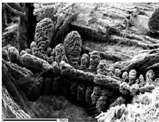
Figure 2 Al dendrite prepared via selective etching
