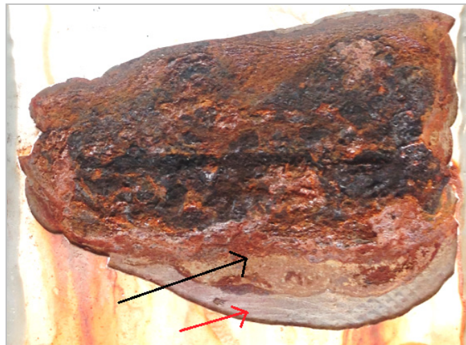
Figure 1: Corrosion creep identified on milled sample C1. Red arrow indicates cathodic disbonding while the black arrow points out the area with corrosion products.
