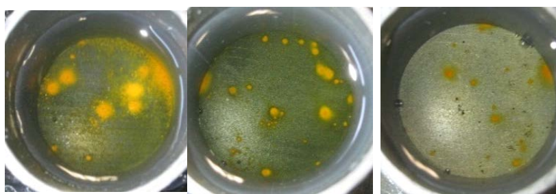
Optical photos of PVB loaded with 2wt% PANI at different doping level after 10 days immersion in 3.5 wt% NaCl solution
