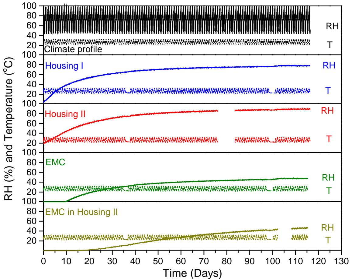
Figure 5: Climate profiles in Housing I, Housing II, EMC and EMC in Housing II exposed to the day/night profile in Jakarta, Indonesia.
