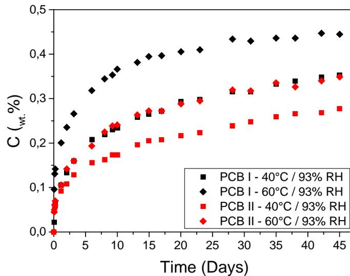
Figure 3: Moisture absorption by the PCB associated with the Housing I and II.
