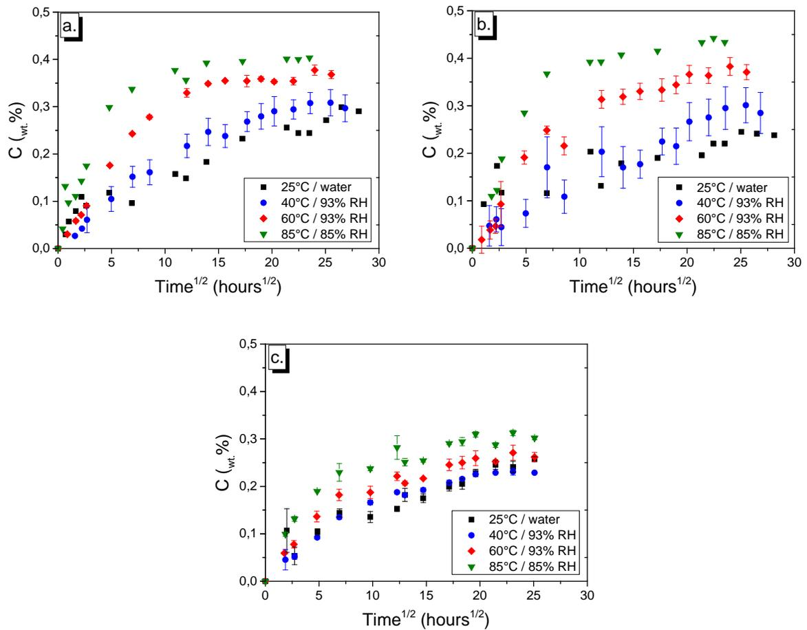
Figure 2: Moisture uptake of PBT: a) with HR and b) without HR, and c) EMC materials.
