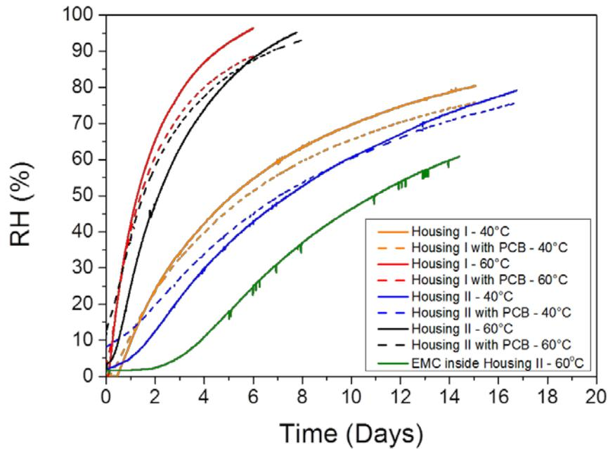
Figure 4: Moisture ingress into the Housing I and Housing II with and without additional components inside at different temperatures and 93% RH.
