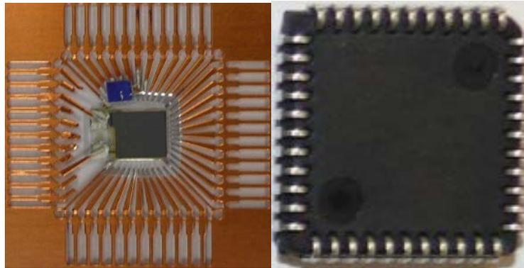
*Figure 1: Pictures of a) Cu lead frame PLCC44 with connected T and RH sensors and b) after molding process of the ECM material.*
