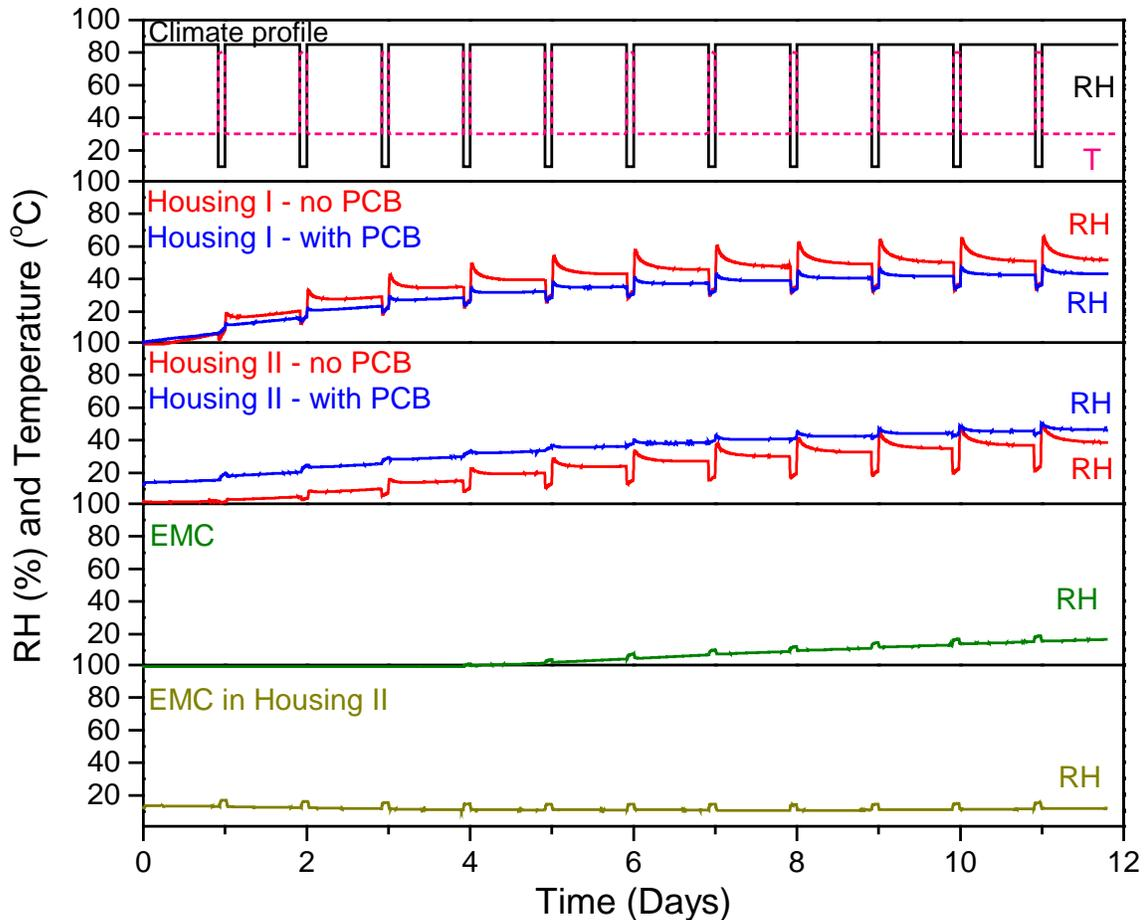
Figure 6: Climate profiles in Housing I, Housing II, EMC and EMC in Housing II exposed to the cyclic conditions: 30 °C / 85% RH / 22 h and 80 °C / 10% RH / 2 h.
