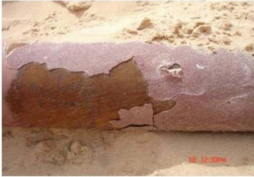
Figure 13: External FBE coating failure on hot flowline (source: NACE Corrosion 2008 Paper 08044).
