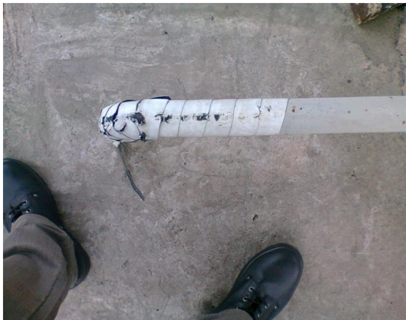
Figure 6: Author inspecting Epoxy Coating on buried gasoline pipeline at the Truck Loading Bay
