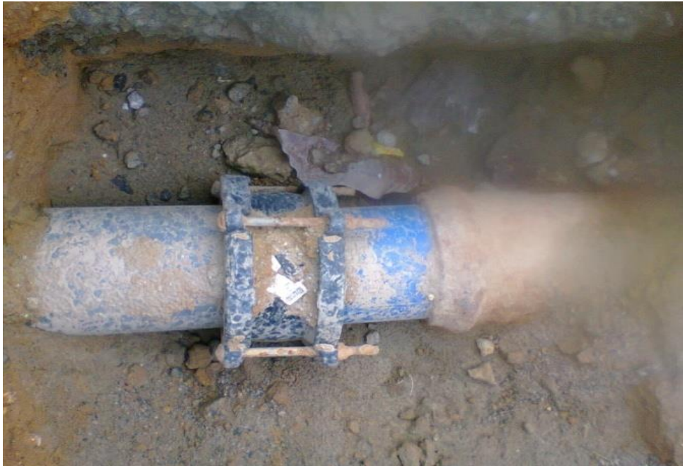
Figure 3: Ruptured Pipeline in the Storage Terminal hitherto monitored offline
