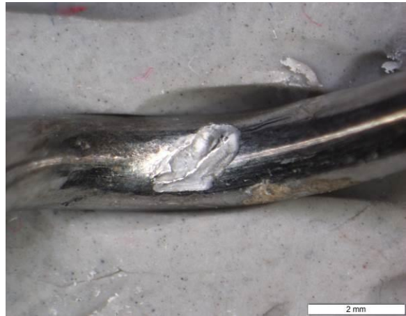
Figure 5 : erosion and corrosion in contact point, 1.4362
