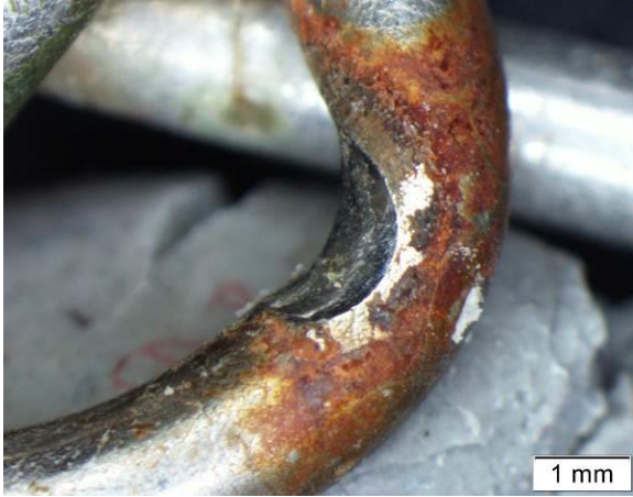
Figure 2 : erosion in contact point
