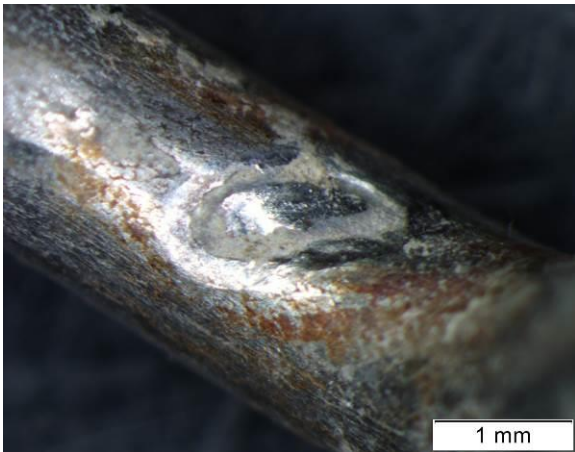
Figure 6 : erosion and corrosion in contact point, 1.4462
