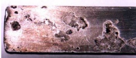
Figure 1. Under deposit corrosion : corrosion pits formed under \text{NH}_4\text{Cl} acidic salt deposits on carbon steel surface (four months) [31].
