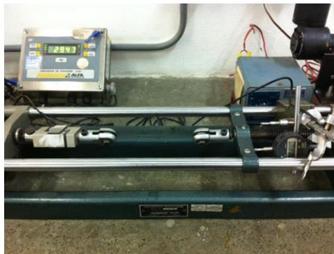
Figure 1 - Horizontal tensile used for the mechanical tests, working length wire of 130mm.
